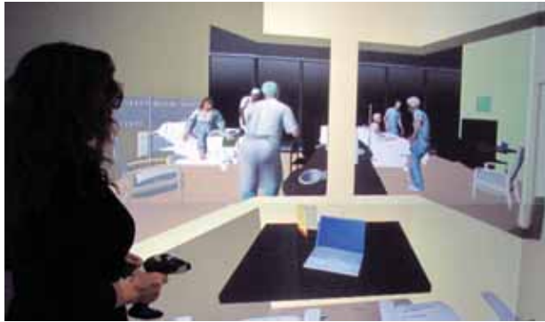
Figure 2: Visuo-acoustic simulations in the CAVE evaluate speech intelligibility of doctors reciting 'sound-alike' medication orders when competing with clinical recordings of conversations, ambient noise, equipment alarms and ventilation sounds
