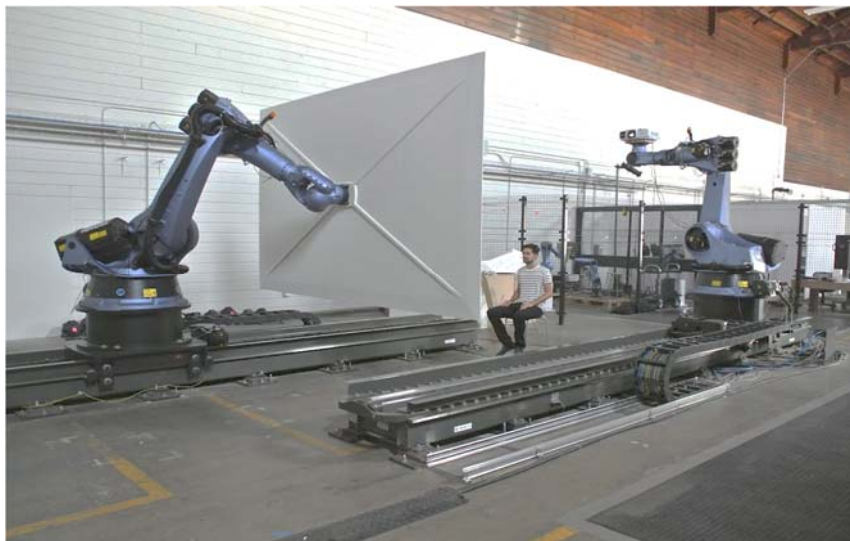
Fig. 3: A setup for measuring solid regions of visibility. A screen and projector are mounted on robotic arms at a fixed distance from one another. An observer facing the screen is seated between the rails carrying the robots. Prompted by periodically acoustic signals, the observer reports his experience in response to visual patterns presented on the screen.
