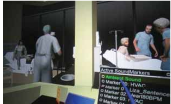
Figure 2: Visuo-acoustic simulations in the CAVE evaluate speech intelligibility of doctors reciting 'sound-alike' medication orders when competing with clinical recordings of conversations, ambient noise, equipment alarms and ventilation sounds
