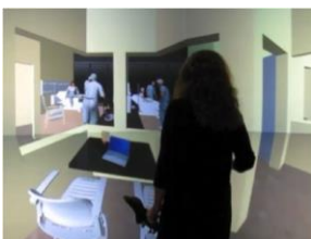
Figure 3. A subject testing visibility of adjacent hospital rooms from a shared nurse's station while testing effects of conflicting sound environments.
