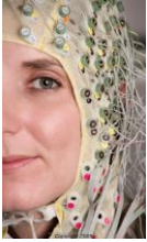
Figure 2. A 256 electrode array records and wirelessly transmits electroencephalographic (EEG) responses.
